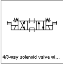
4/3-way solenoid valve with bypass position
