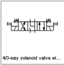
4/3-way solenoid valve with floating position
