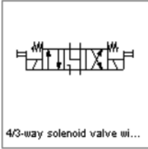
4/3-way solenoid valve with floating position
