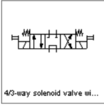
4/3-way solenoid valve with bypass position
