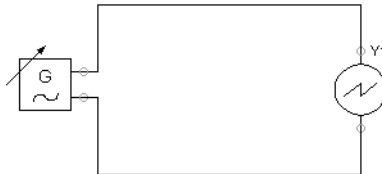
Figure 9/45: Simple circuit with function generator and oscilloscope
