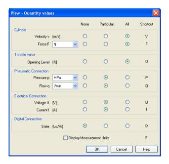
For each of the listed quantities ("Velocity", "Pressure", ...) a display mode can be chosen.
