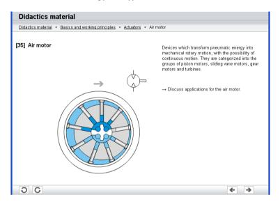
Often it is easier to understand the functional nature of a component, when its behavior is visualized through the use of animation. For this reason, several components possess different sectional views showing the component at different states. These sectional views can be animated in much the same way as a flip book.
