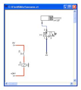
Aside from a manual or electrical operation, valves can be controlled *mechanically*, either through a cylinder piston or a magnet mounted at the piston. Such a coupling is realized in the same way an electrical coupling is established: By means of labels, which are assigned to the cylinder's distance rule and the mechanical valve connection.
