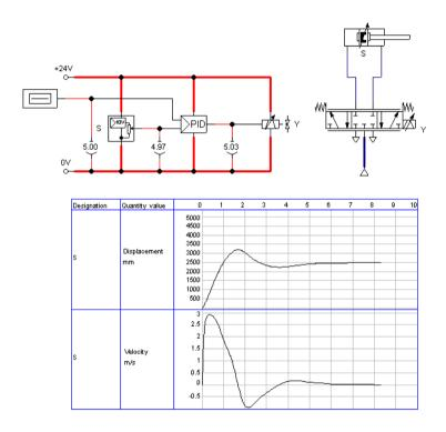
It often may be desirably to make a cylinder travel by maximum speed until it reaches its desired position, and to make it stop most spontaneously. To achieve this we can amplify the position signal of the displacement encoder and therefore accelerate the reversing of the control valve. In doing so we make use of the fact that the PID-controller limits the output voltage of the proportional valve magnet to 10 volts.
