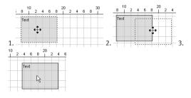
A double-click on a text box in the edit mode opens a corresponding dialog box. You can adjust the representation of the text box with it.
