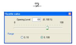
To help with precision adjustment some controllers provide an optional control range. You may alternatively enter the numeric value using the input field.
