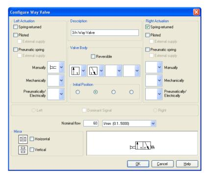
Double click the valve to assign an operation mode to it. A dialog box appears:
