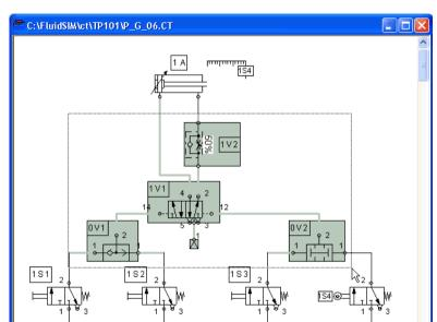
All components enclosed, either partially or fully, by the rubber band, are selected.
