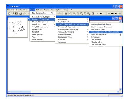
After a symbol has been chosen, it is inserted in the current diagram and gets selected. It then can be moved and connected as usual.
