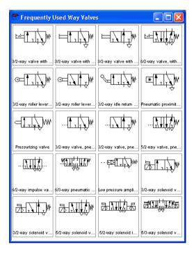
Inserting Components Via Menu In FluidSIM, several alternative concepts exist to insert a component into a circuit diagram. One concept is "Drag-and-Drop", which has been used in the preceding examples.
