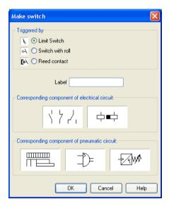
This means that there do not exist special symbols for these switches in the FluidSIM component library. Instead the symbols for simple switches can be utilized:
