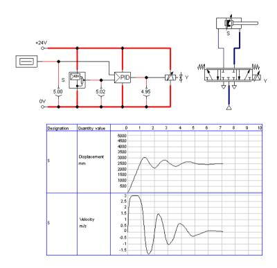
It is clear that cylinder now travels at a constant speed over a long distance. It will then be firmly slowed down and will finally stop completely.
