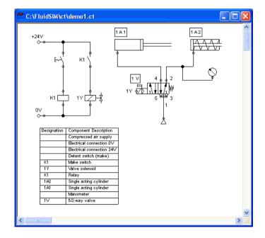
The parts list component analyzes all components of the diagram and generates table with columns for the component identifications and the component designations. In this connection, FluidSIM uses existing labels and texts as component identifications.
