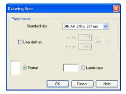
The size and the orientation of the paper can be set here. If the drawing size exceeds the paper size of your printer, the total area of several smaller papers can be tiled with the drawing.
